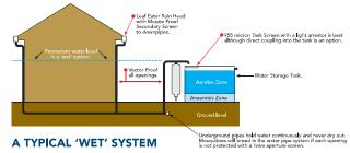
A 'wet' system is a system where the pipes are fitted in such a way that when the rain stops the pipes do not drain out. They hold water. With this type of system, the pipes must be fitted with screens at each end to ensure that vectors (mosquitoes etc.) cannot enter and breed within the system.
